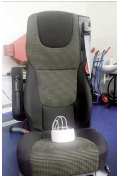
Fig. 10. Portable measuring device on a real car seat
